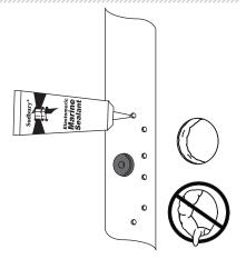
Insert the black nylon shoulder washers into the correct holes on the mast mount feet. Use the supplied rivets to secure the mast mount to the mast.
