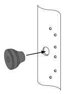
Put some marine adhesive sealant into the holes. Do not apply too much sealant.
